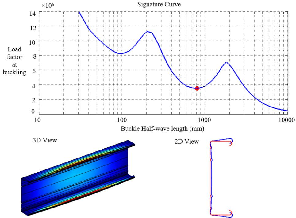
c) The distortional buckling mode under the bending in the positive direction
