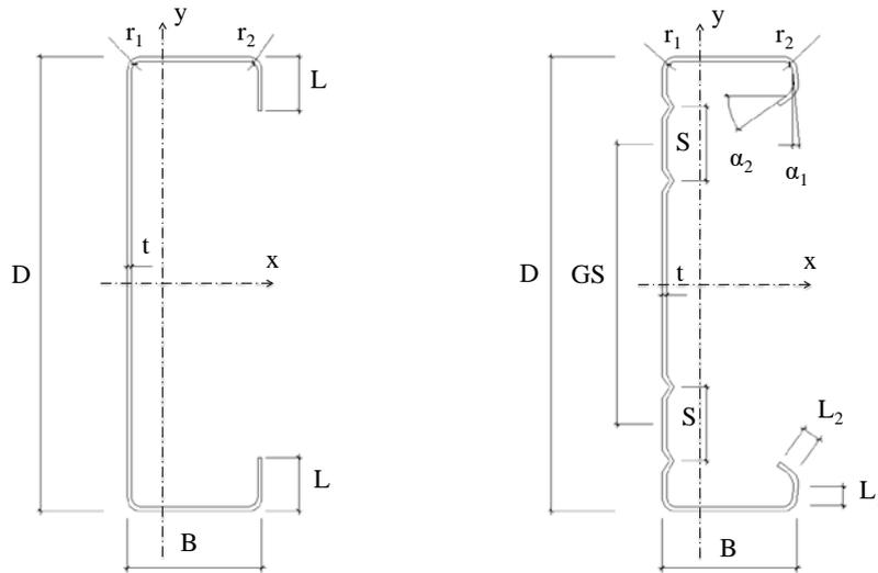
Fig.1 Nomenclature for channel and SupaCee sections
