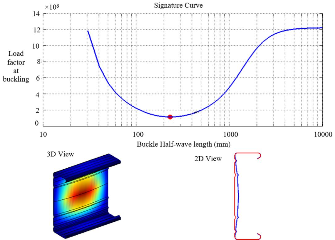
a) The local buckling mode under the bending in the negative direction
