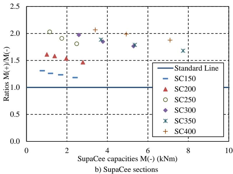
Fig.5 The ratios  $M^{(+)} / M^{(-)}$  for channel and SupaCee sections
