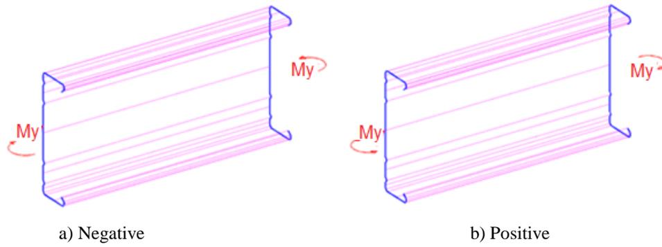
Fig.2 The illustrations of bending directions
