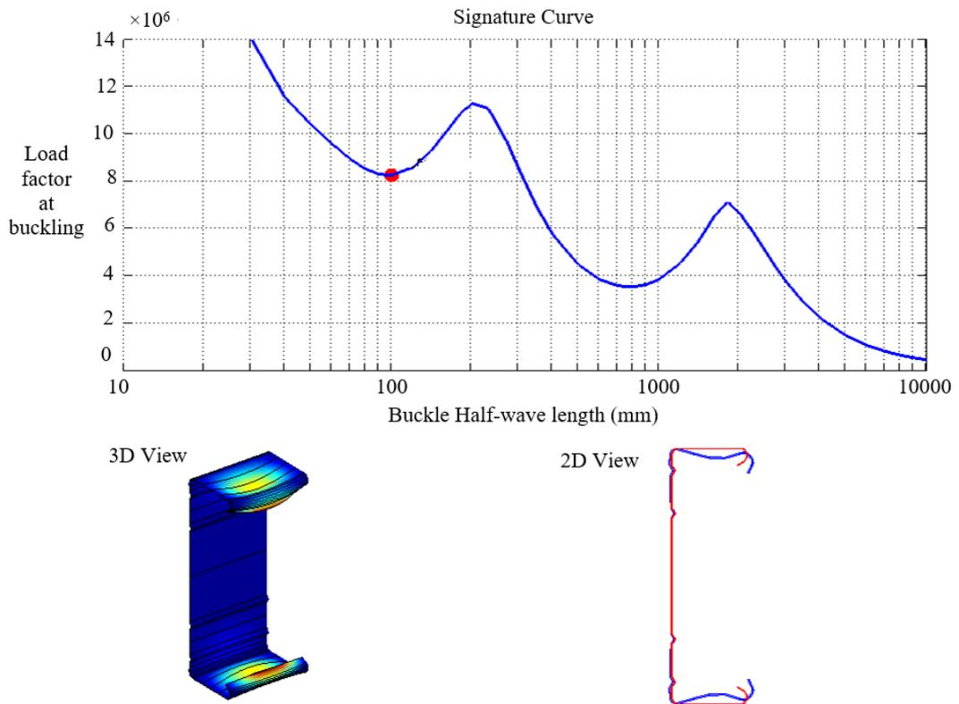
b) The local buckling mode under the bending in the positive direction
