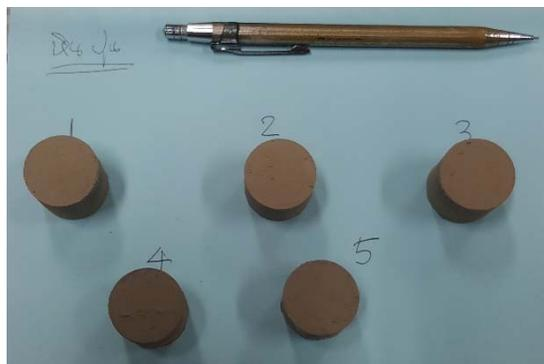
(b) Sample briquettes extruded from the mold
