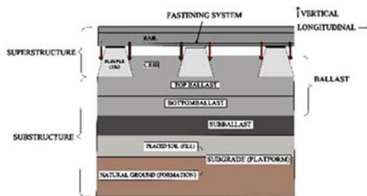
Fig. 2 Railway track structure components [2]
