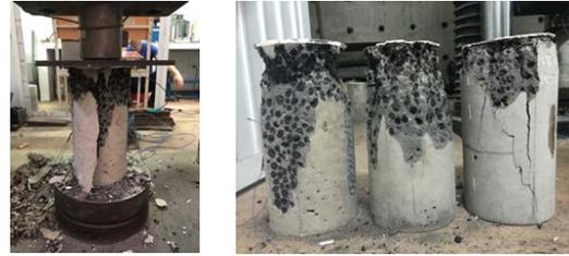
Fig.6 The failure mode of cylinders in tests of modulus of elasticity
