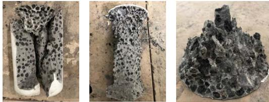
Fig.2 The failure of cylindrical specimens for compression tests
