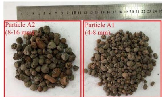
Fig.1 Recycled LWA made from CDW
