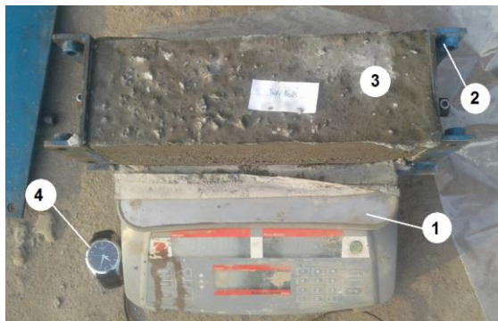
Fig.5 Illustrates the process of measuring the water loss of concrete
