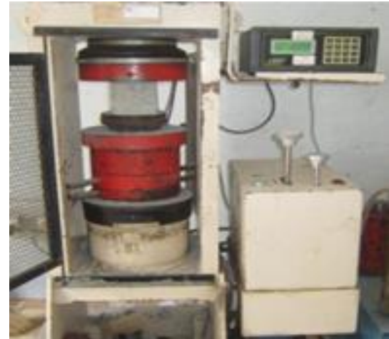
Fig.9 Compression of samples to determine strength
