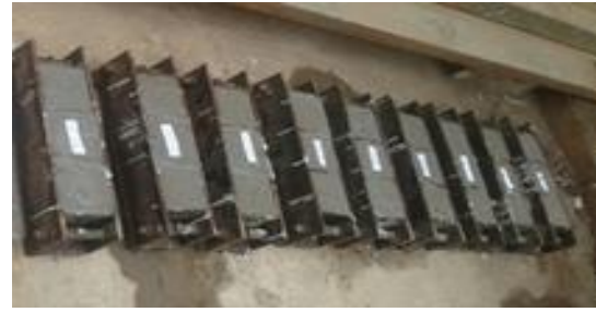
Fig.8 Casting samples to determine strength ( R^{28} )
