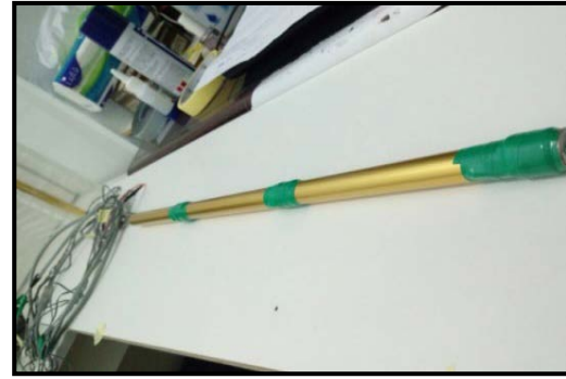
(a) Locations of strain gauges and load cell on the pile
