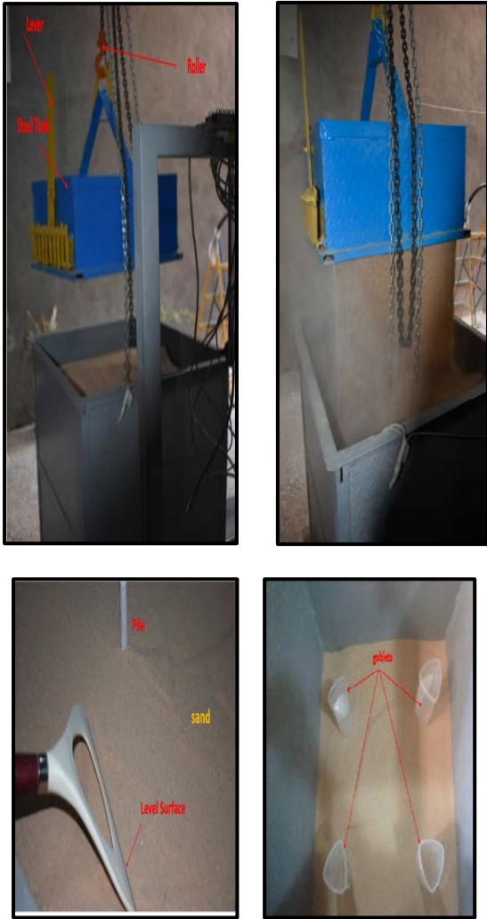
(e) the raining technique Fig.4. Saturation system and the raining technique
