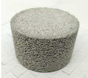
Fig. 1 Pervious mortar filter with a diameter of 8.2 cm and a thickness of 5 cm.
