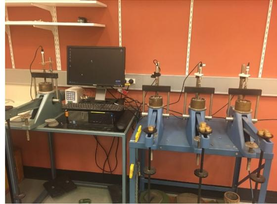
Fig. 2 Conventional Oedometer Apparatus
