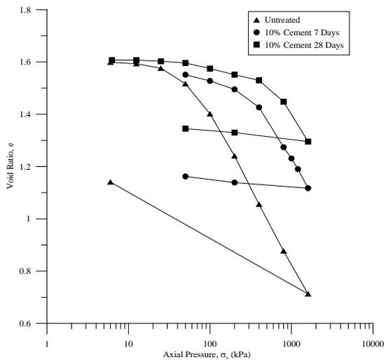
Fig. 3 Typical e-log P Curves of Cement Treated SEQ Soft Soils
