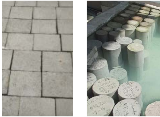
Fig.1 Concrete bases (left) and test cylinders (right)
