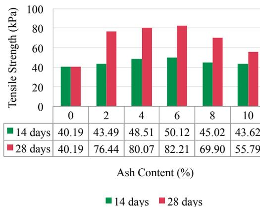
Fig. 8 Effect of ash content on the tensile strength of mixed soil with 14 days and 28 days of curing
