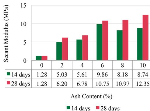
Fig. 7 Effect of ash content on the modulus secant of mixed soil with 14 days and 28 days of curing
