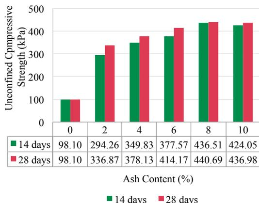
Fig. 6 Effect of ash content on the unconfined compressive strength of mixed soil with 14 days and 28 days of curing
