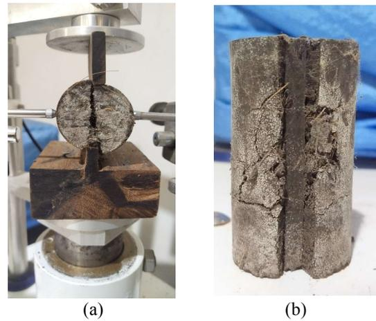
Fig. 3 (a) Tensile strength test (b) Specimen after testing.
