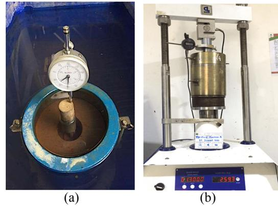
Fig. 1 (a) Swelling test (b) CBR test
