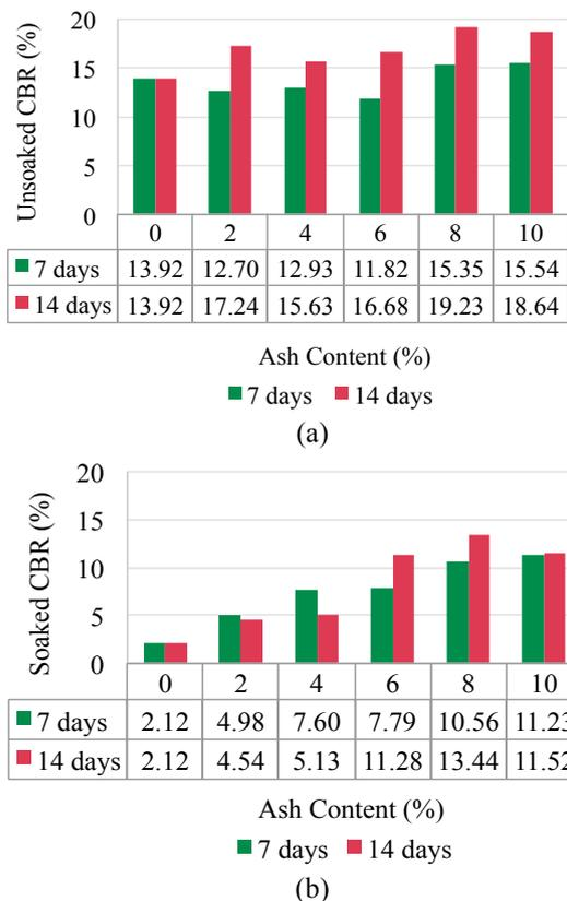
Fig. 4 Effect of ash content on the CBR of mixed soil with seven days and 14 days of curing (a) unsoaked CBR, (b) soaked CBR
