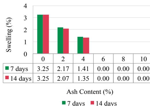
Fig. 5 Effect of ash content on the swelling of mixed soil with seven days and 14 days of curing
