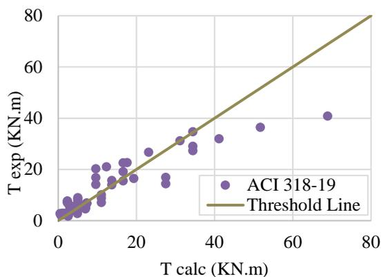
Fig.6 Experimental versus analytic torsional strength (ACI 318-19)
