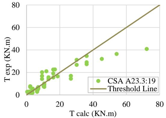
Fig.7 Experimental versus analytic torsional strength (CSA A.23.3:19)
