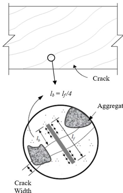
Fig.4 Steel fiber tensile stress mechanism
