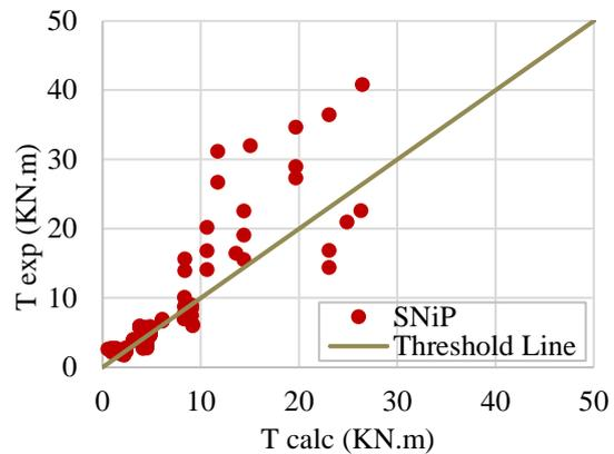
Fig.8 Experimental versus analytic torsional strength (SNiP)
