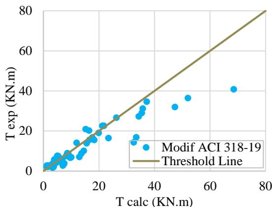
Fig. 10 Experimental versus analytic torsional strength (ACI 318-19 Modification)
