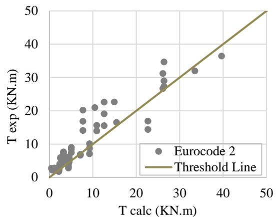
Fig. 9 Experimental versus analytic torsional strength (Eurocode 2)
