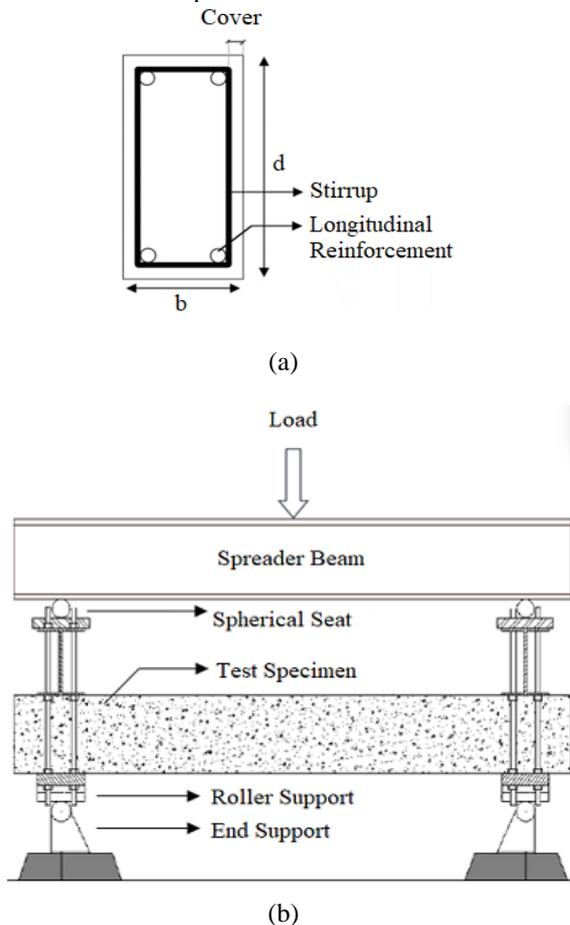
Fig.1 Illustration of the test setup and loading beam
