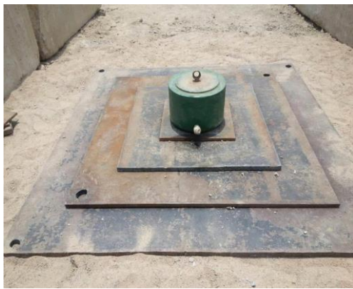
Fig. 3: Large plate load test on CFA piles and surrounding soil.
