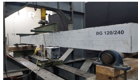
Fig. 2 Two-Point Load Test Setup
