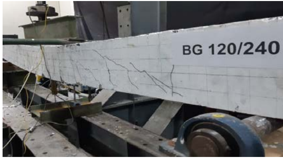
Fig. 10 Geopolymer R/C Beam (BG 120/240), Post-Loading
