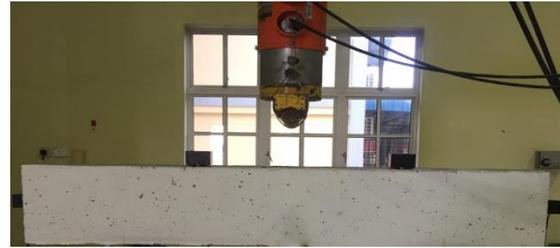
Fig.2 Experimental set-up with three-point flexural testing.
