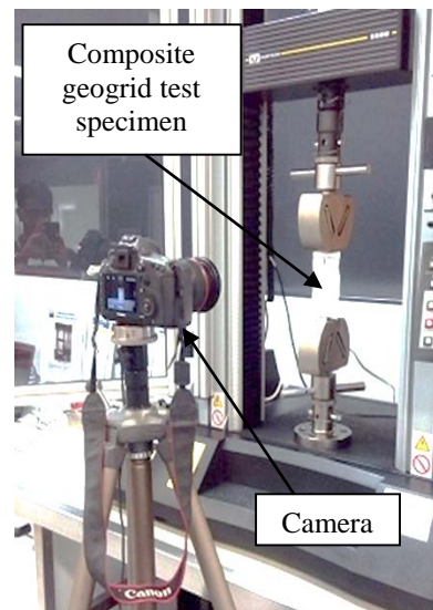
Fig.6 Taking photographs for PIV analysis
