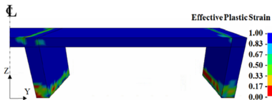
Fig. 17 Effective plastic strain in concrete (EQ2)
