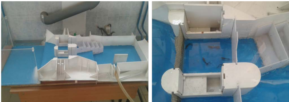
Fig. 6. Laboratory layout of a fish-passing facility 1:100
