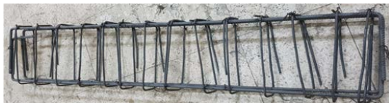
Fig.1 Geometry and steel reinforcement for tested beam
