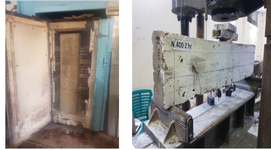
Fig. 3 Furnace and loading test setup
