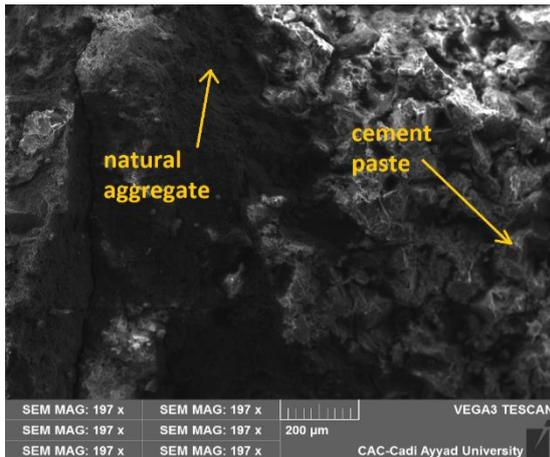
Fig.13 SEM images of the two types of concrete after 28 days of curing of the conventional concrete.
