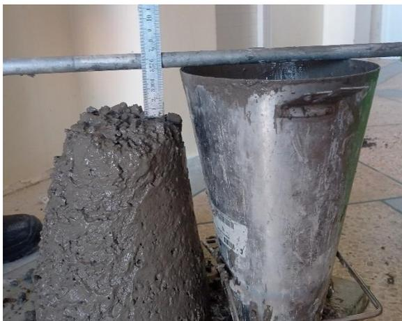
Fig.5 Illustration of slump measurement.
