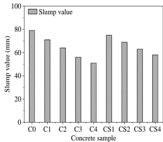
Fig.6 Slump values of concrete samples.
