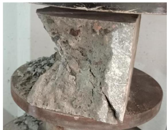
Fig.7 Rupture pattern of concrete specimens under compression.
