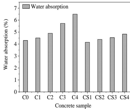
Fig.12 Water absorption of concrete samples.
