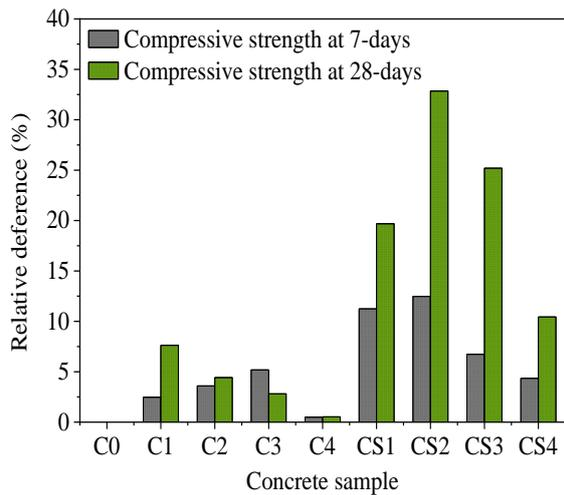
Fig.9 Relative difference of compressive strength at 7 and 28 days.
