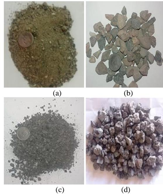
Fig.1 a) Natural sand (NS), b) natural crushed aggregate (NCA), c) Steel slag fine sand (SSf), d) Steel Slag aggregate (SSA).
