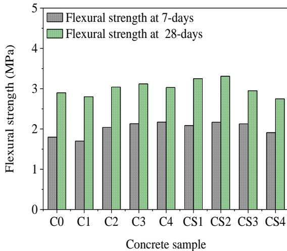
Fig.10 Flexure strength of concrete mixes types at 7 and 28 days.
