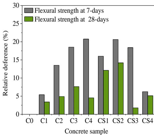
Fig.11 Relative difference of flexure strength at 7 and 28 days.
