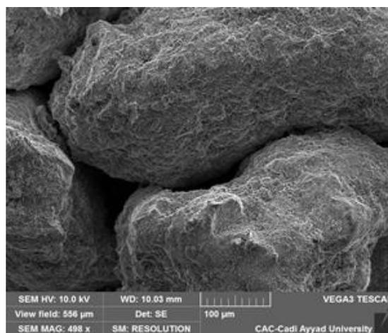
Fig.2 SEM analysis of steel slag.
