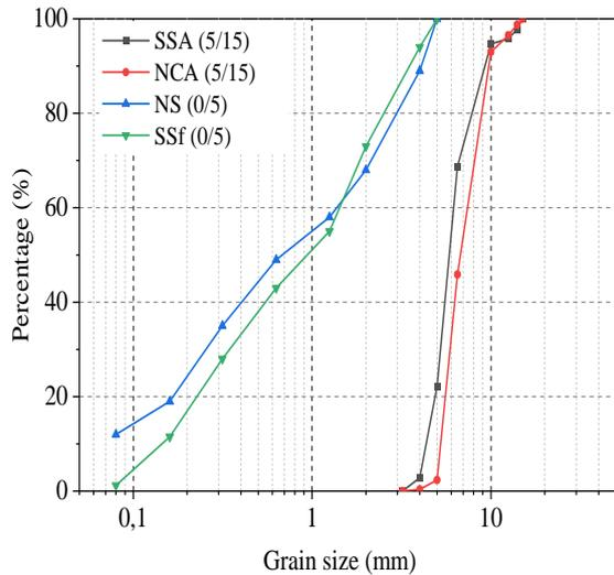
Fig.3 Particle size distribution of the materials used.
