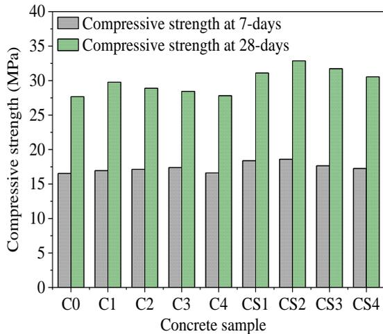
Fig.8 Compressive strength of concrete mixes at 7 and 28 days.
