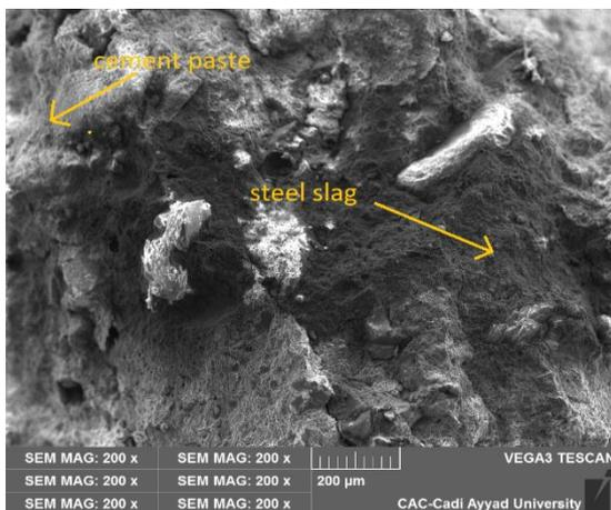
Fig.14 SEM images of the two types of concrete after 28 days of curing of concrete made of steel slag.
