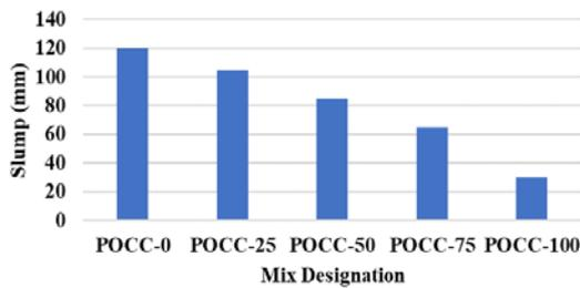
Fig. 2. The slump of geopolymer concrete mixtures at different POCA percentages
