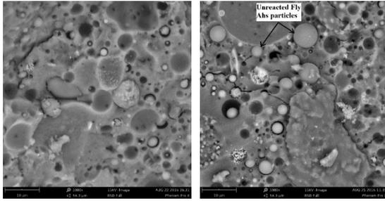
Fig. 7. SEM micrographs of POCC-0 (left) and POCC-100 (right) cracked specimens
