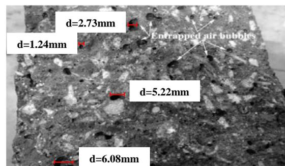
Fig. 6. The fractured surface of POCC-100 mixture specimen
