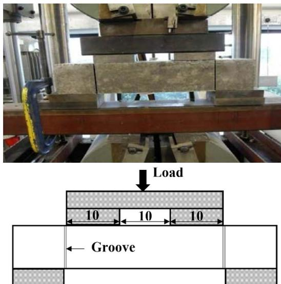
Fig. 1. Direct shear test setup
