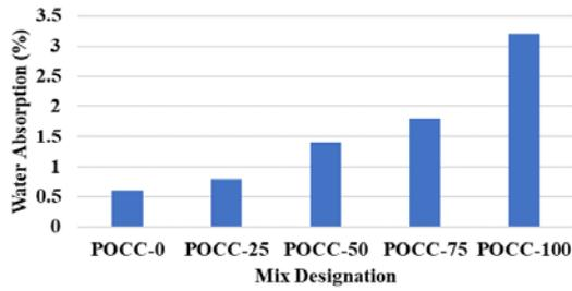
Fig. 3. Water absorption of geopolymer concrete mixtures at different POCA percentages
