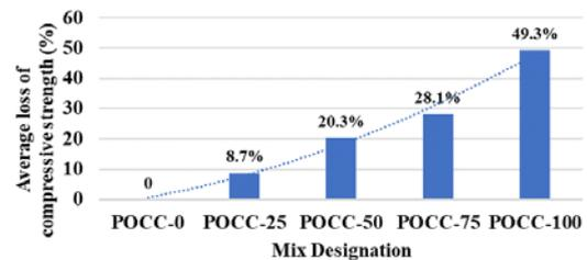
Fig. 5. Average compressive strength loss at the age of 90 days of different mixtures
