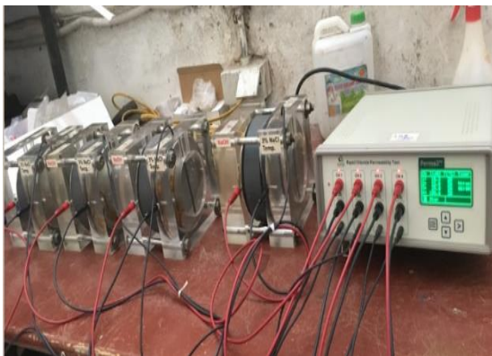
Fig.5 The experiment for measuring chloride ion permeability through concrete
