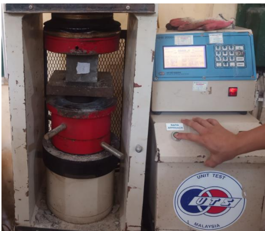
Fig.3 The compression test of concrete samples
