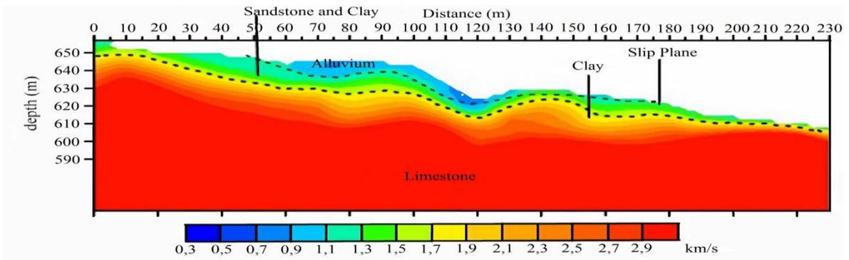
Fig. 5 Seismic Refraction Result at L2
