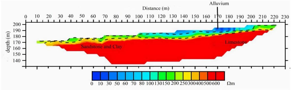
Fig. 4 Resistivity Results at L1
