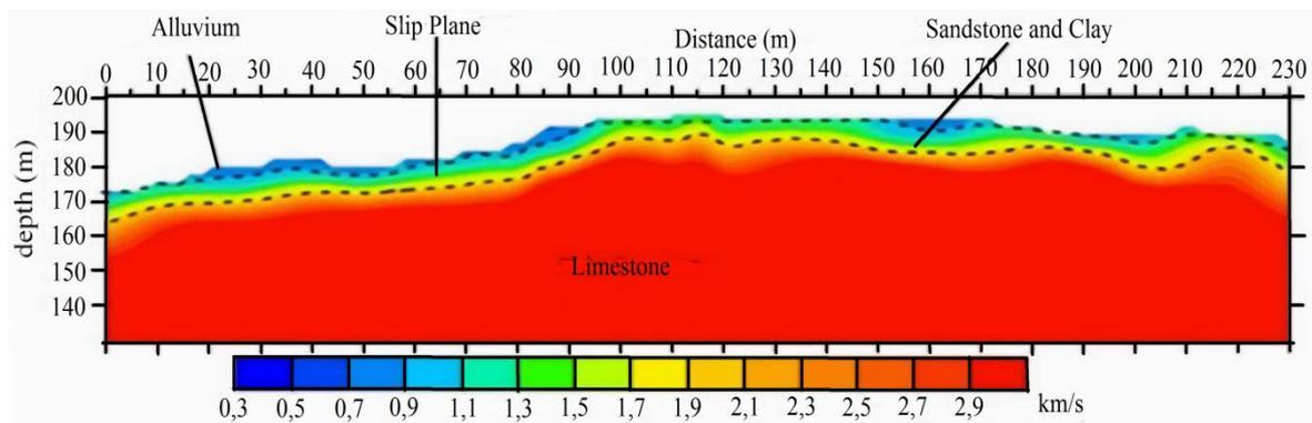
Fig. 3 Seismic Refraction Results at L1
