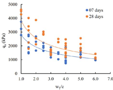
Fig.6 Relationship between  $q_u$  and  $w_T/c$  at 7, 28 days curing
