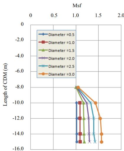
Fig.20 The FS of the road foundation along the Cho Gao canal at E=75 MPa
