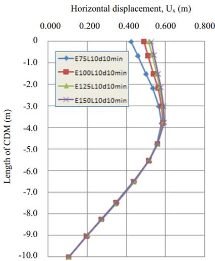
Fig.19 Horizontal displacement of CDM columns when changing Young's modulus
