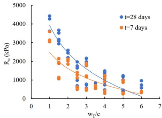
Fig.11 Relationship between  $R_u$  and  $w_T/c$  at  $t=7, 28$  days curing
