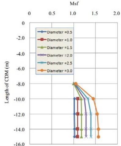
Fig.21 The FS of the road foundation along the Cho Gao canal at E=150 Mpa
