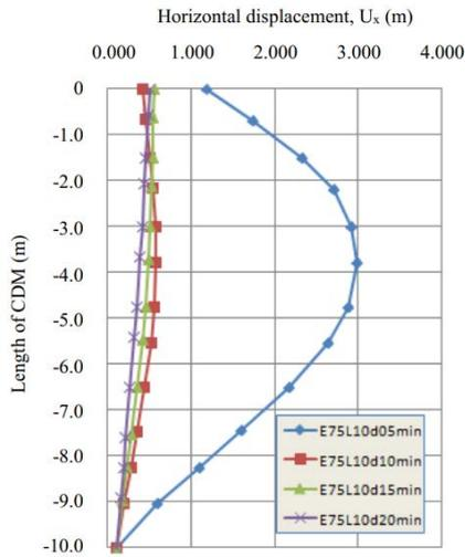
Fig.18 Horizontal displacement of CDM columns when changing diameter
