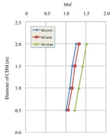
Fig.17 Factor of safety when changing the water level and diameter of CDM columns
