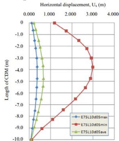
Fig.16 Horizontal displacement of CDM columns when changing water level
