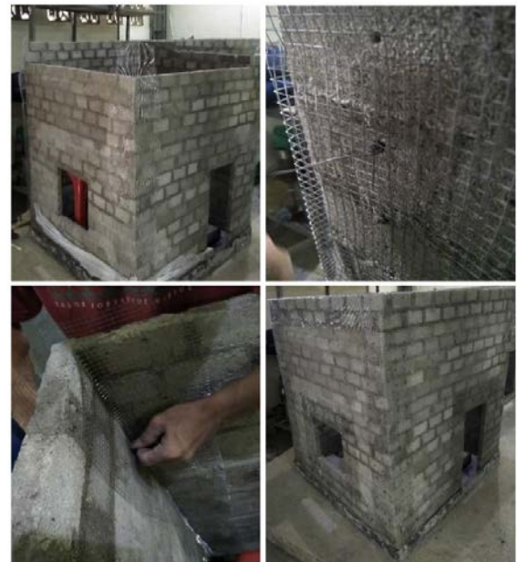
Fig.13 Repair of the concrete crack and installment of woven wire in the damaged B1 specimen
