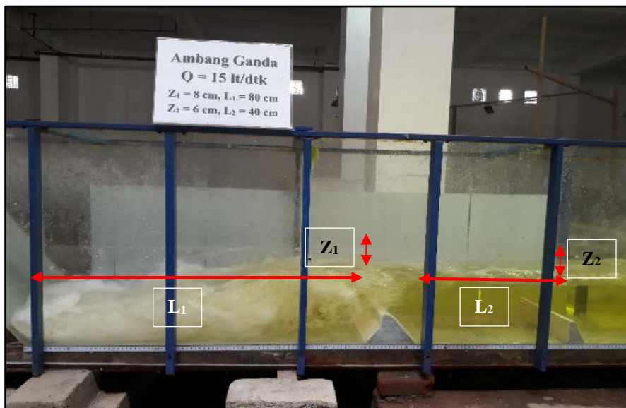
Fig. 5 Sketch depiction of double sill research hydraulics model test
