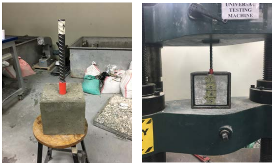
Fig. 1 Concrete cube sample under pull out test
