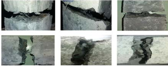
Fig. 5 Fiber failure mode of tensile strength specimens
