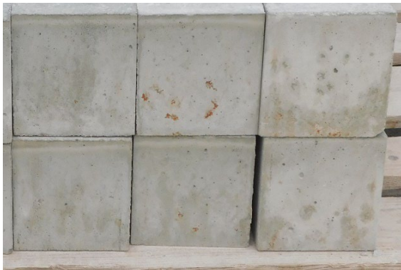
Fig. 3 Sample specimens with discoloration due to chemical attack after being embedded in natural soil.
