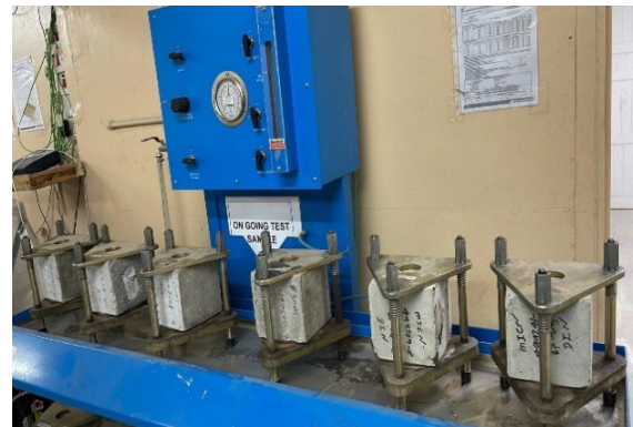
Fig. 7 Water penetration of the hardened concrete test setup.
