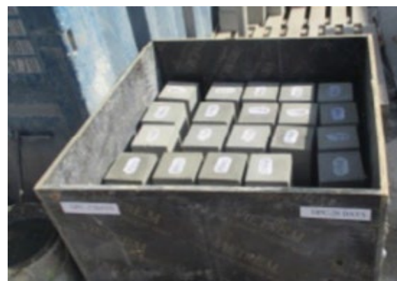
Fig. 1 Sample specimen before being embedded in natural soil.
