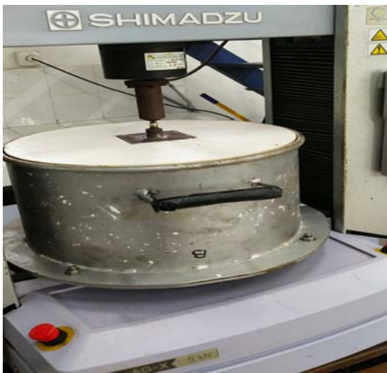
Fig.14 Position of the specimen for the soil shear failure test.
