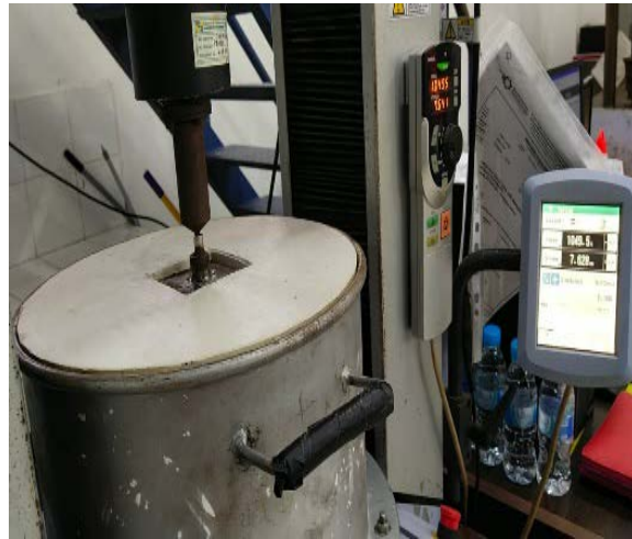
Fig.16 Shear failure test of soil when the settlement was approximately 0.1B .
