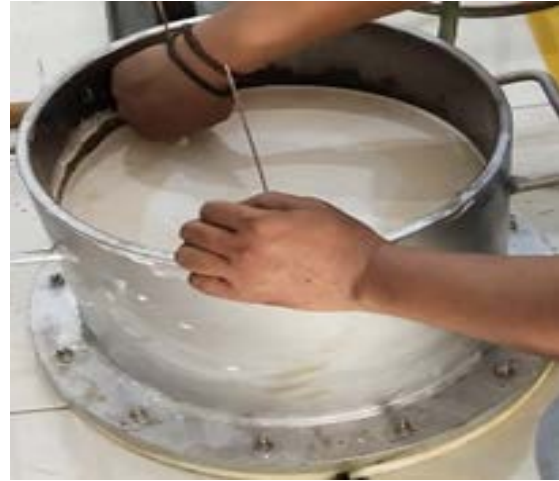
Fig.10 Measurement of the compressed slurry sample height ( H_1 ) with a soft clay load ( \sigma_p' ) of 114.149 kN/m 2 .
