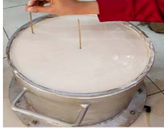
Fig.9 Measurement of the slurry sample height ( H_0 ) to be compressed.
