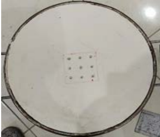
Fig.12 H_{sc} specimen with several micro-piles n_2= 9 and configuration K_1 .
