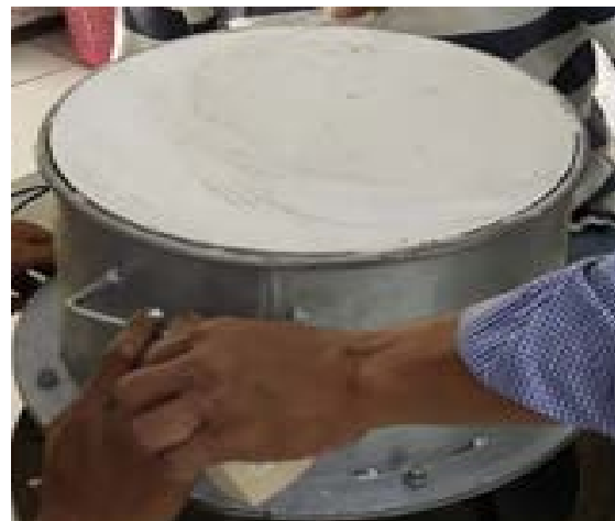
Fig.11 Cutting soft clay soil ( H_1 ) in the test specimen tube with a height ( H_{sc} ) of 0.185m.
