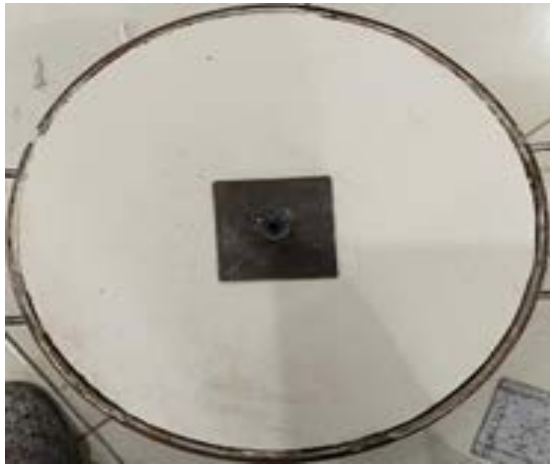
Fig.13 H_{sc} test specimen installed on a plate foundation on micro-piles.
