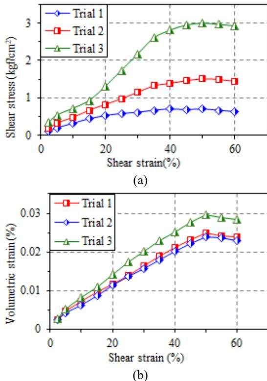
Fig. 5 Shear Stress vs. Shear Strain (a) & Volumetric Strain vs. Stress Strain (b) of 60M40A Mix.
