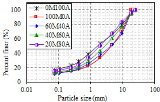
Fig. 4 Comparison of grain size distribution curves of each mix proportion
