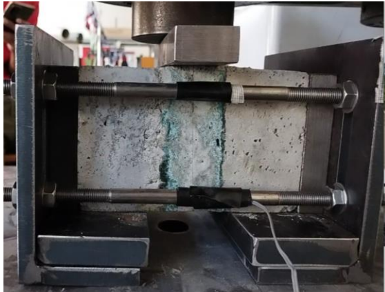
Fig. 9 Double shear strength test
