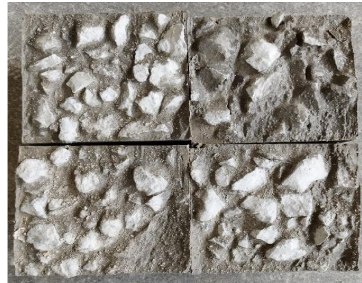
Fig. 6 Surface roughness preparation for double shear test
