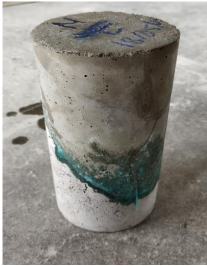
Fig. 3 Slant shear sample
