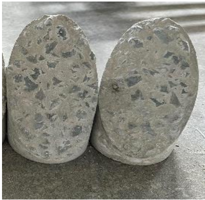
Fig. 5 Surface roughness preparation for slant shear test
