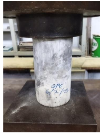
Fig. 8 Slant Shear experiment
