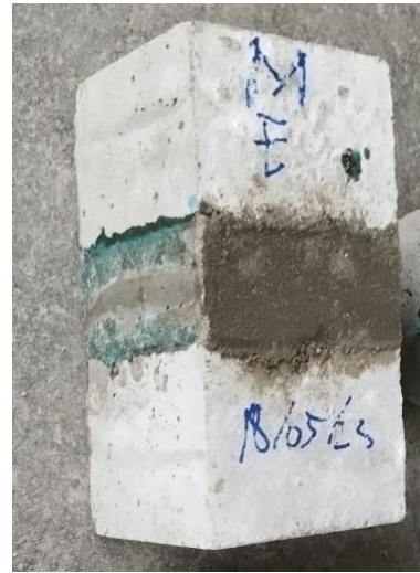
Fig. 4 Double shear sample
