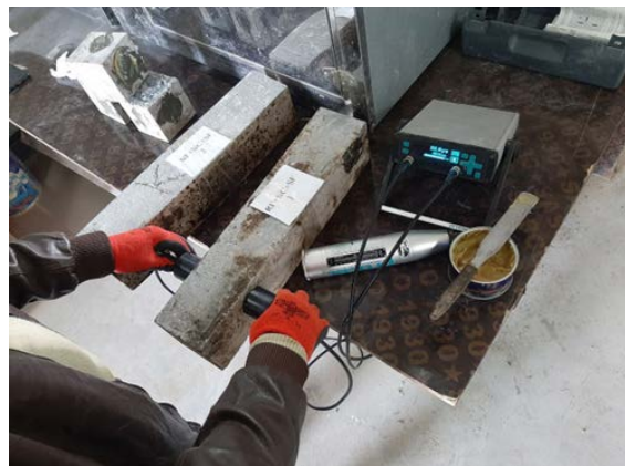
Fig. 7 Rebound hammer test
