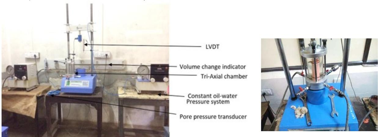
Fig.4 Triaxial cell apparatus and specimen prepared on the cell
