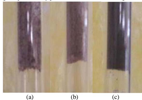
Fig.5 Test tube showing (a) Perfect arch in fine sand (b) Partial arch in silt (c) No arch in clay
