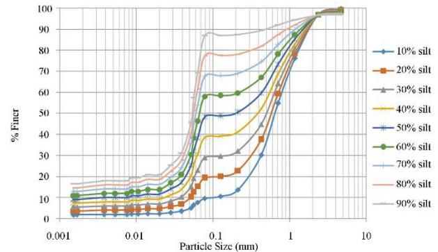
Fig.1 Grain Size Distribution curve for sand-silt mixtures
