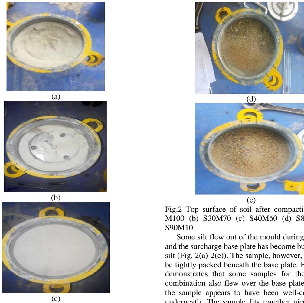
Fig.2 Top surface of soil after compaction for (a) M100 (b) S30M70 (c) S40M60 (d) S80M20 (e) S90M10
