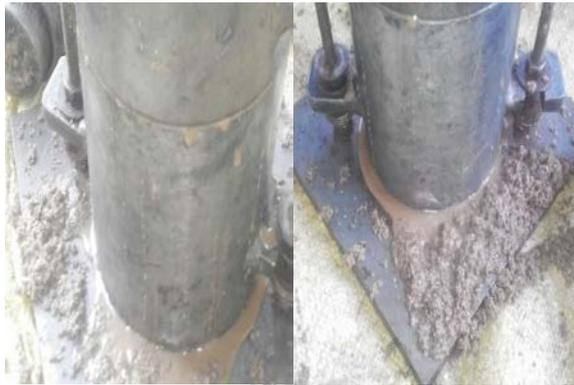
Fig.3 Expulsion of water from the mould during proctor compaction test
