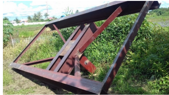
Fig.4 Loading frame from welded steel
