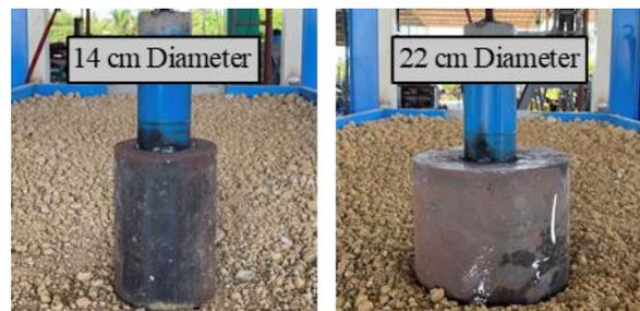
Fig. 3 Two different sizes of the cylindrical plunger.
