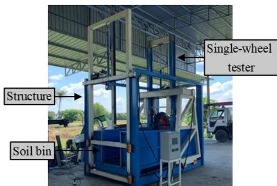
Fig. 2 The developed tire testing machine.
