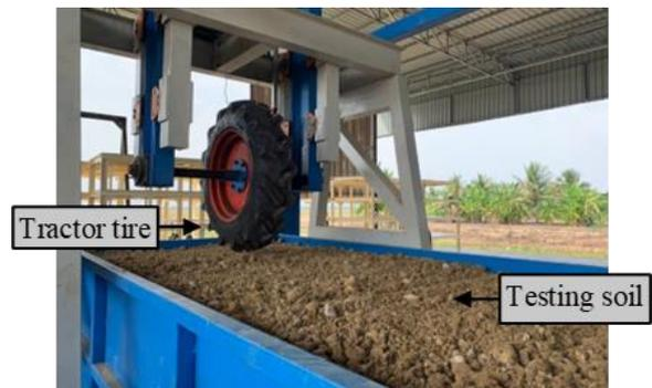
Fig. 6 Tractor tire mounting on the TTM.
