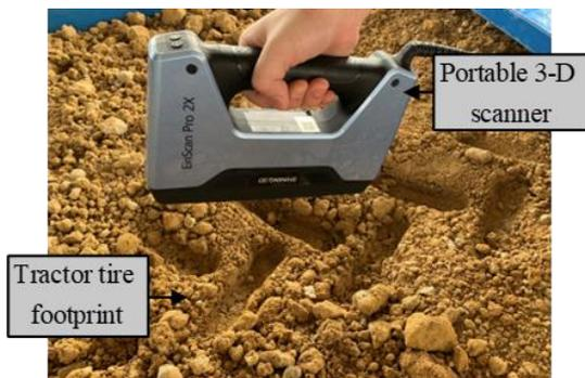
Fig. 9 3D scanning of the tractor tire footprint
