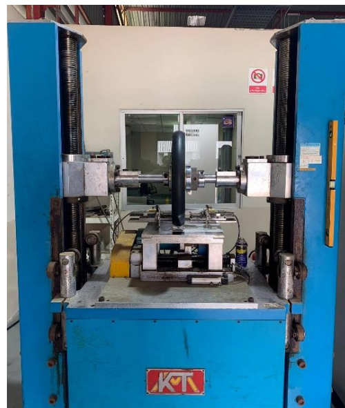
Fig.1 Mounting of a smooth tread motorcycle tire on the tire testing machine
