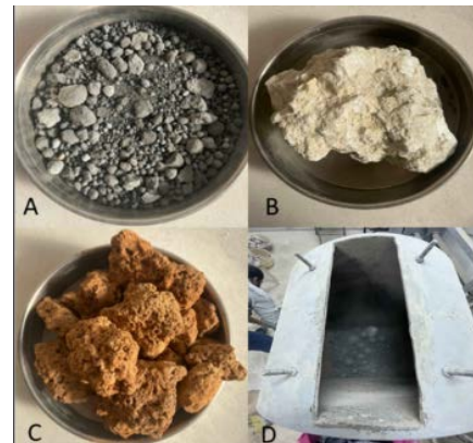
Fig.1 Shows: (A) clinker, (B) Gypsum, (C) natural zeolite, (D) ball mill used in grinding of zeocement.
