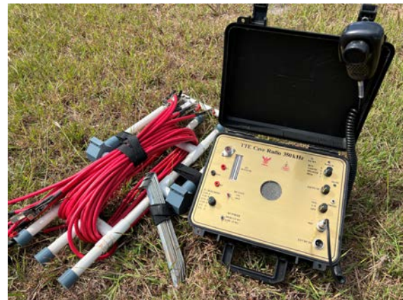
Fig.17 Prototype of TTE 350 kHz cave transceiver
