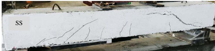
(a) Beam SS (with stirrups and without SFs)
