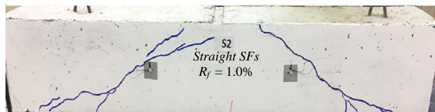
(c) Beams S2 (with 0.5% straight SFs)
