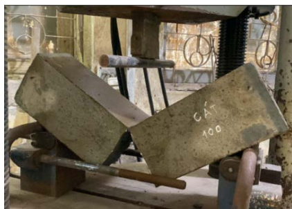
(a) RFA 100 Flexural Test
