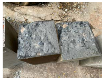
(b) Cross-sectional damage of RFA 100 specimen
