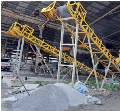
Fig.1 Recycling process of RFA from waste concrete in Hanoi
