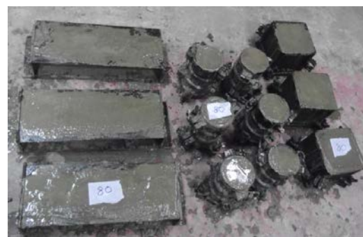
Fig. 3 Concrete casting in molds
