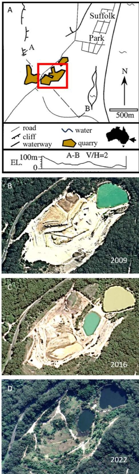
Fig. 1 Example of some stages that may occur in extraction and back-filling. Batson's Sand and Gravel quarry, northern New South Wales
