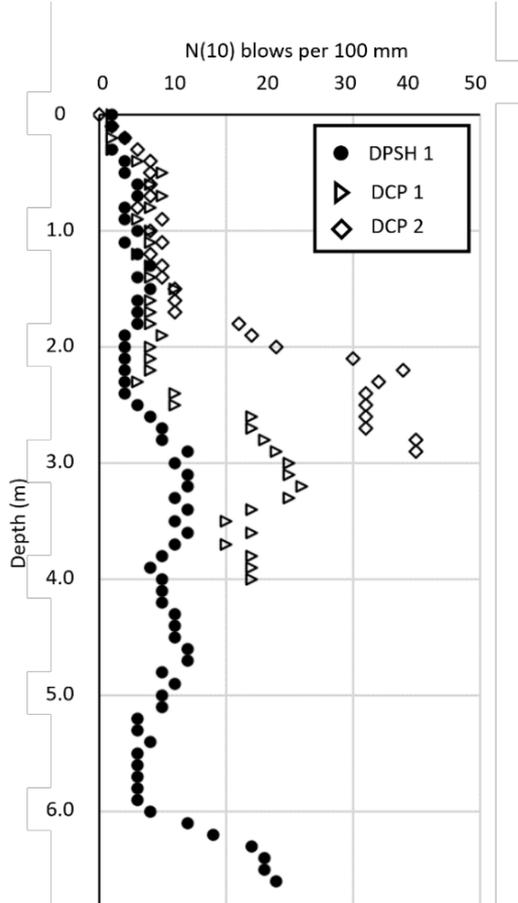
Fig. 7 Graph of one DPSH and two DCP field tests in sand. DCP 1 terminated at the target depth, and DCP 2 met refusal. Full depth of DPSH 1 is not shown
