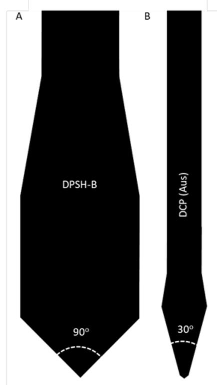
Fig. 3 Illustration of the (A) DPSH and (B) DCP (Australian) dynamic cone heads and shafts to relative scale
