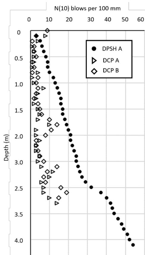
Fig. 8 Graph of one DPSH and two DCP field tests in a constructed clay batter. DCP A and DCP B were terminated at refusal. Full depth of DPSH A is not shown.
