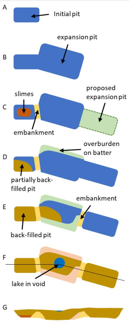
Fig. 2 Illustration of some stages that may occur in extraction and back-filling. A-F: plan view. G: cross-section of stage F
