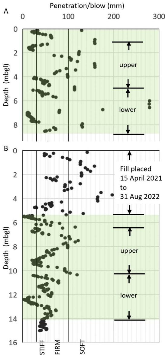
Fig. 4 Graphs of DPSH penetration per blow values (A) before and (B) after placement of approximately 5 m of fill. Shaded area shows the interval of overlap of the before and after probes separated into arbitrary upper and lower zones for comparison in Table 2
