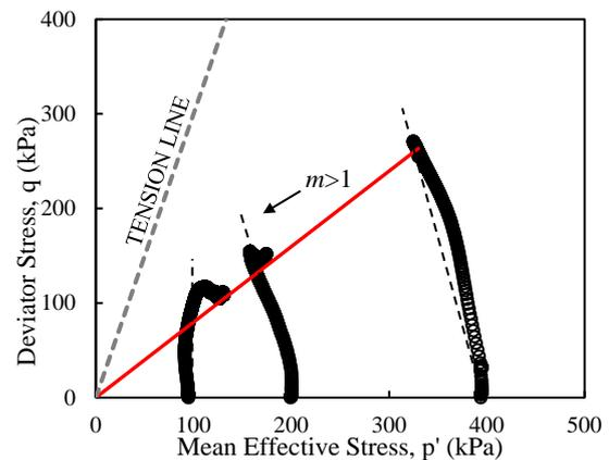
Fig.8 Clay blanket CIU triaxial test results.
