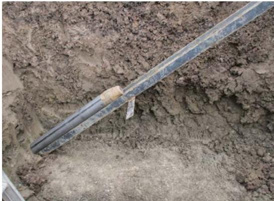
Fig.1 Shelby tube clay foundation sample with inclined orientation
