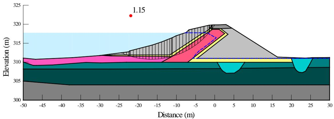
Fig.13 Slope stability analysis for Section B using Case 2.
