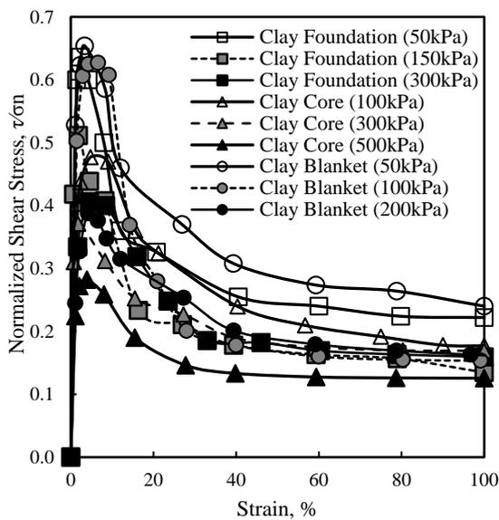
Fig.10 Stress-strain behavior from CD direct shear tests.
