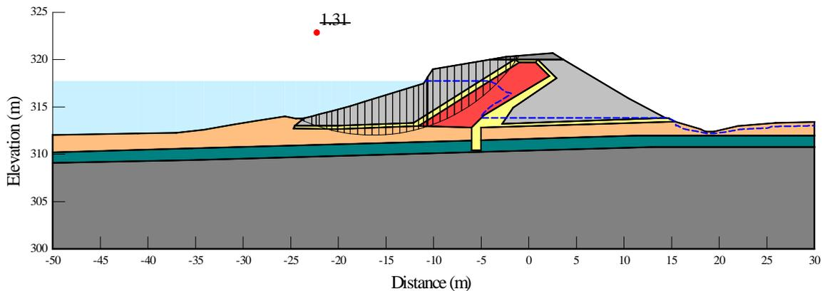
Fig.10 Slope stability analysis for Section A using Case 1.
