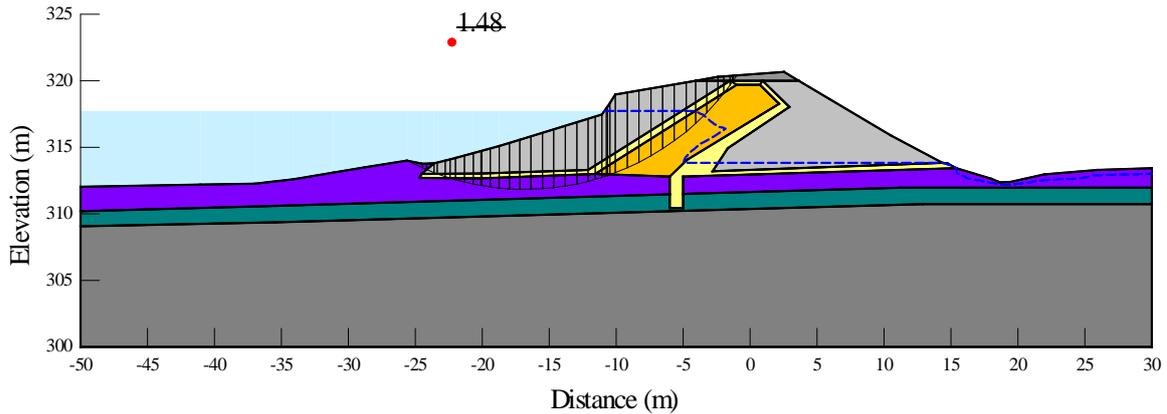
Fig.12 Slope stability analysis for Section A using Case 2.
