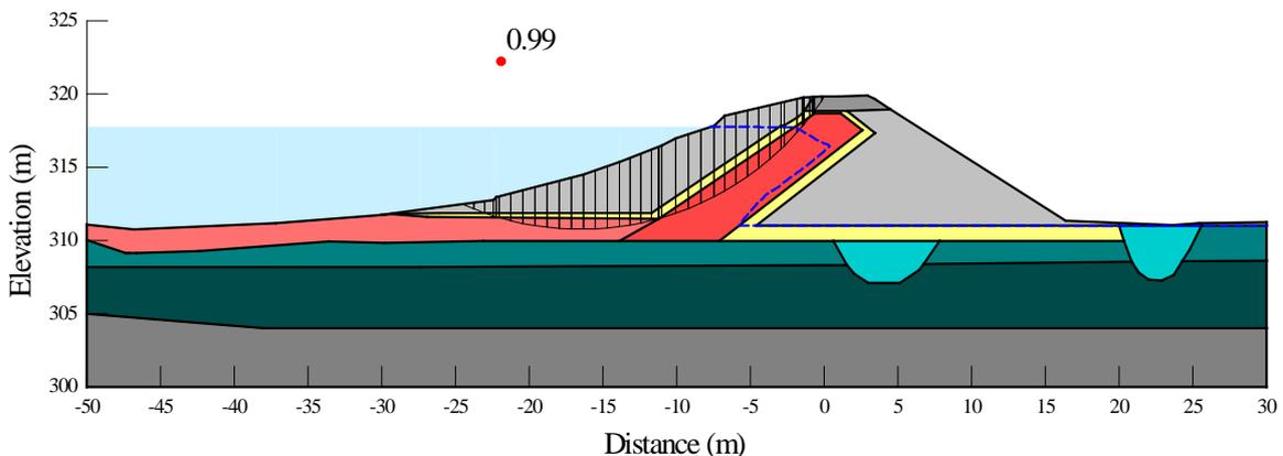
Fig.11 Slope stability analysis for Section B using Case 1.
