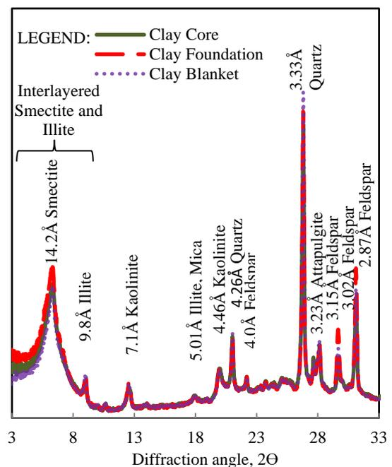
Fig.6 XRD results from clay core, blanket, and foundation.
