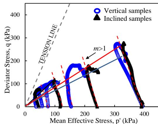
Fig.9 Clay foundation CIU triaxial test results.
