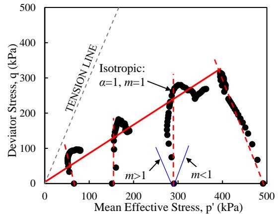
Fig.7 Clay core CIU triaxial test results.
