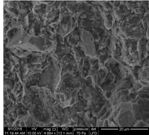
Fig.5 SEM image of clay foundation.
