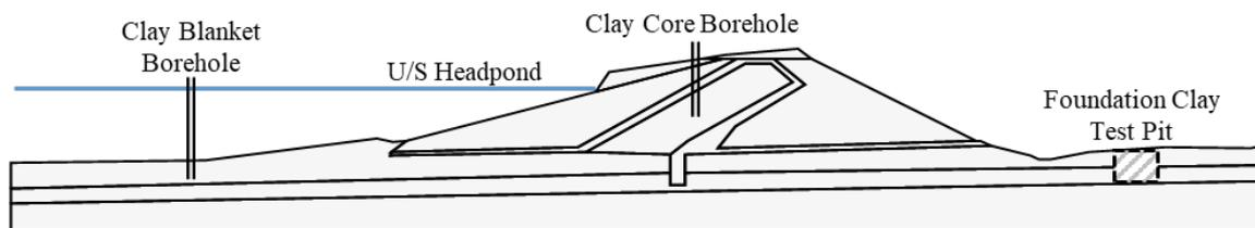
Fig.2 Typical borehole and test pit sampling locations
