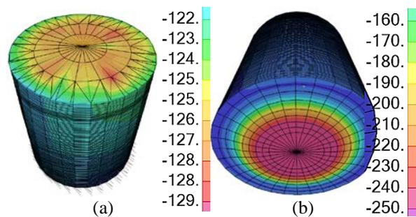
Fig.8 Tank deformation (a) roof view (b) base view
