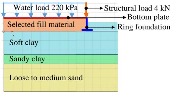
Fig.3 Root cause analysis axisymmetric model
