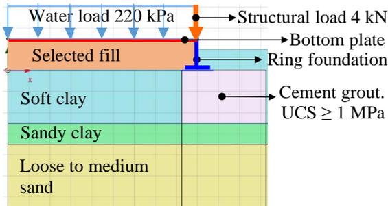
Fig.5 Retrofit by cement grouting scheme
