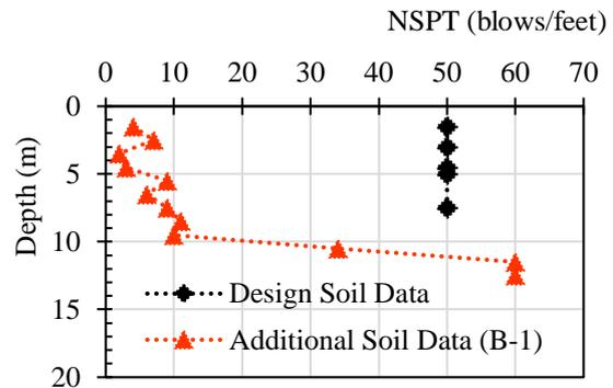
Fig.2 Existing and additional soil data
