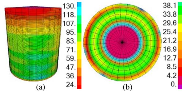
Fig.9 Tank Von Mises stress contour (a) wall (b) base
