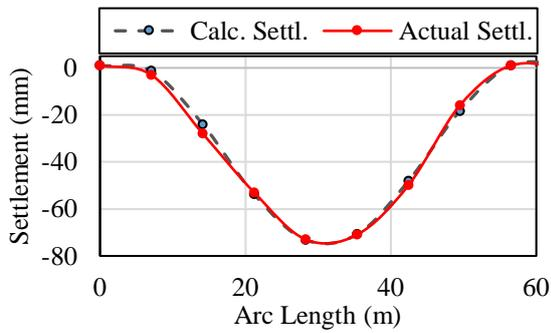
Fig.4 Tank perimeter settlements - actual vs planar
