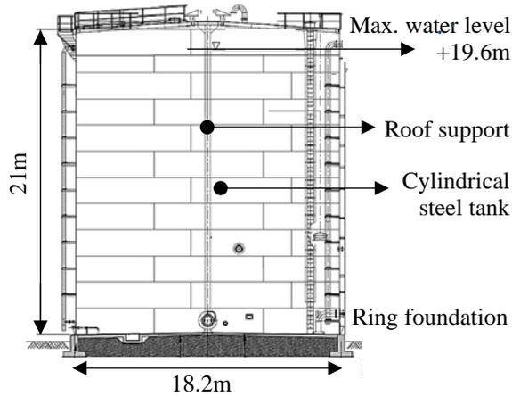
Fig.1 Firefighting - steel water tank at Cilegon
