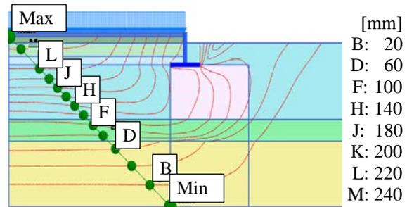
Fig.7 Potential max settlement of improved soil
