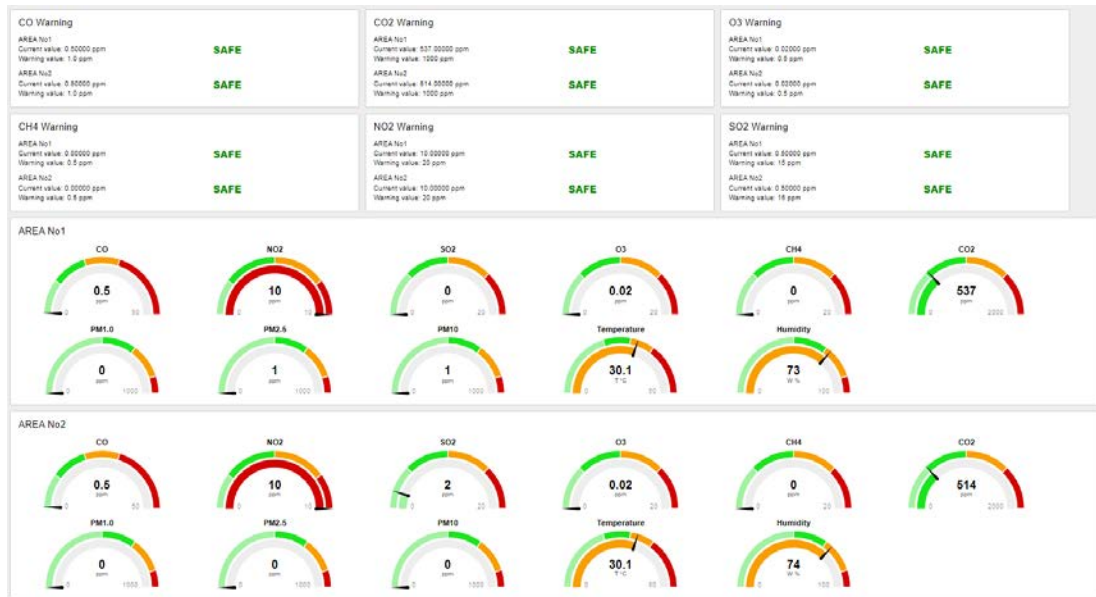
Fig. 11 Warning interface of the measuring system
