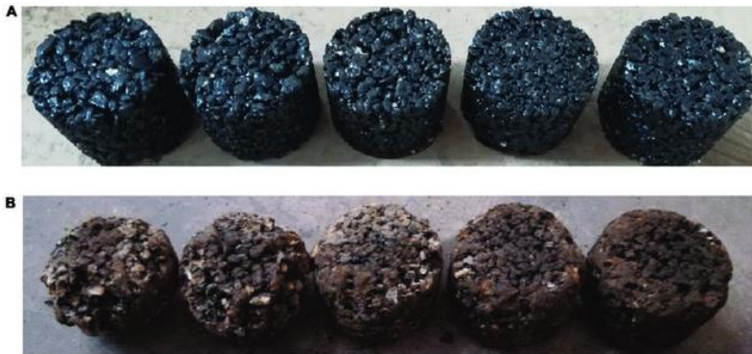
Fig. 5 Specimen morphology following an abrasion loss test (A. Before testing, B. After testing)
