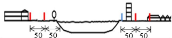
Caption | Placement of portable weather station | Placement of temperature/RH data logger (a)
