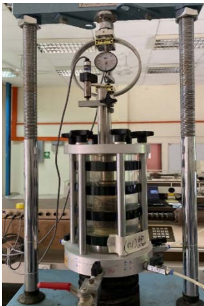
Fig.2 Triaxial Test – Unconsolidated Undrained Set Up
