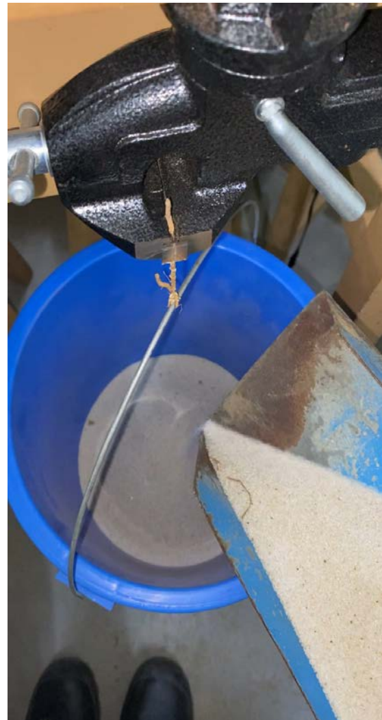
Fig. 2a Modified Grass Root Tensile Test Machine
