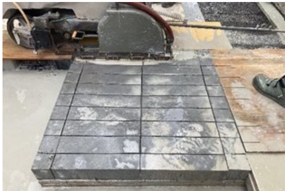
Fig. 3 Prism specimens cut from the square slab
