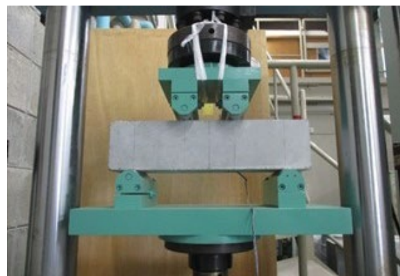
Fig. 5 Four-point flexural fatigue test setup
