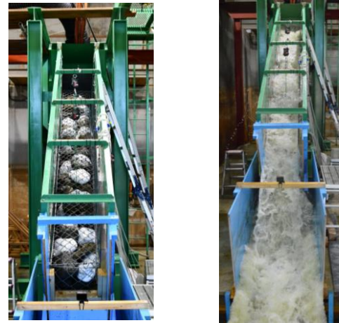
(a) Top surface of gabion packed with rock particles (b) Overtopping flow in 0.5m-wide sloping water flume
